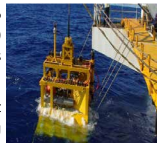
Remotely Operable In-situ Soil Tester (ROSiS)
