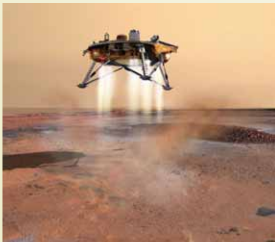
Fig. 1. This artist's concept depicts NASA's Phoenix Mars Lander a moment before its 2008 touchdown on the arctic plains of Mars. Pulsed rocket engines control the spacecraft's speed during the final seconds of descent. (Image credit: NASA/JPL-Caltech/University of Arizona)
