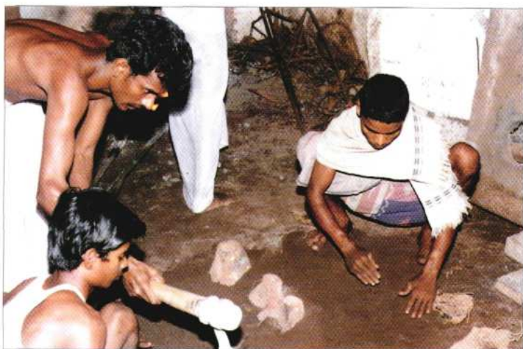
Pl. 3.11 The red hot pre-heated mould is buried under the ground with its mouth open
