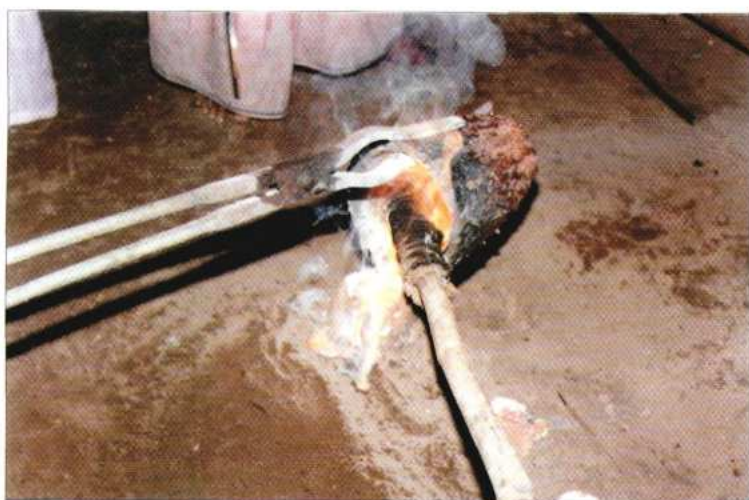
Pl. 3.12 The molten alloy is poured inside the red hot buried mould
