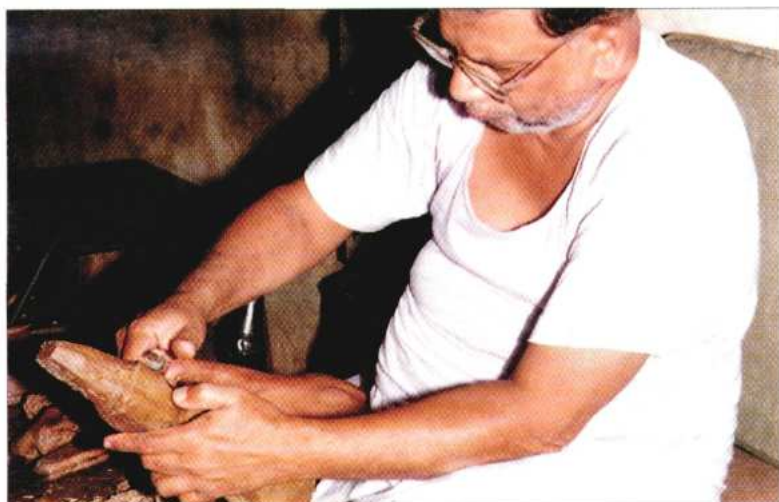
Pl. 3.2 Shaving off excess wax from various parts of the Icon
