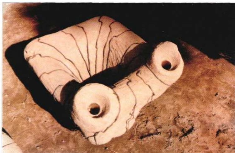
Pl. 3.7 The mould from which wax is removed (note the iron wires that strengthen the mould)
