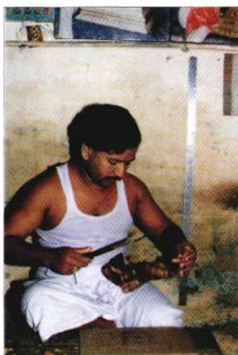
Pl. 3.4 Fixing the limbs(made separately) with the torso of the wax model
