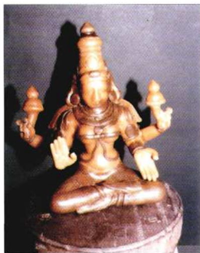
Pl. 3.5 A complete basic wax model ready for clay coating
