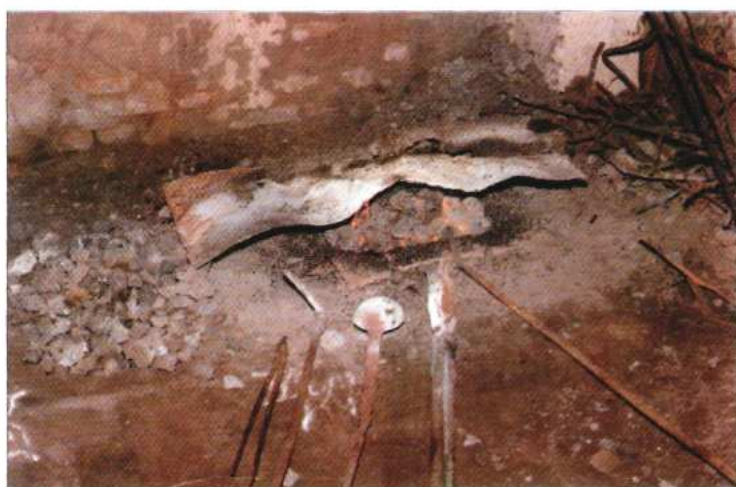
Pl. 3.10 Various tools used during melting of alloy (tools for holding the crucible, mixing the alloy)
