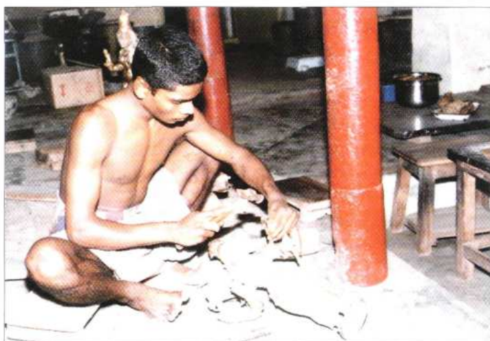
Pl. 3.13 The icon, obtained after breaking the mould, is worked with to bring out the finer features
