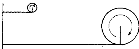
A larger wheel covers a larger distance in one revolution.
