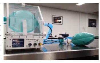
optimized for an application which regulates the airflow mechanism, collects the data from pressure sensor and uploads it to the cloud. The estimated cost of the Ventilator will be Rs. 3000-4000, in comparison to the commercial ones, which are currently priced at Rs. I.5 lakh.
