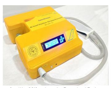
SwasthVayu BiPAP machine in Auto Test mode with Test Lung
